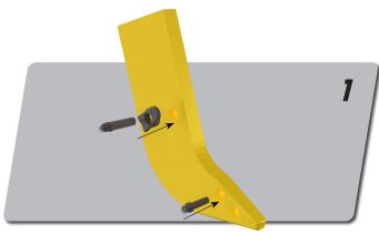
Insert converter into upper retainer hole and place guard lower pin in the lower retainer hole.
