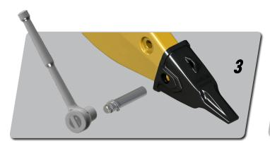
Insert helical pin and rotate 180 degrees with a socket wrench to engage lock.
