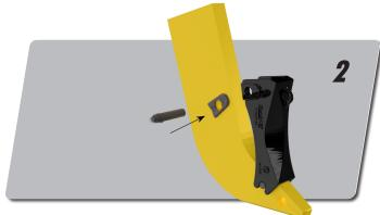
Rest protector slot onto the guard lower pin.
