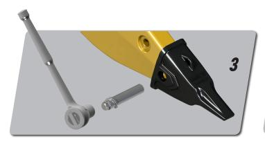
Insert helical pin and rotate 180 degrees with a socket wrench to engage lock.
