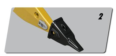
Fit tooth over nose and converter.
